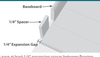
Leave at least 1/4" expansion spaces between flooring and ALL vertical objects (walls, cabinets, pipes, etc.) Large flooring runs may require additional expansion space. Undercut door jambs and casings to provide adequate expansion space. Bamboo Design does not recommend screwing or nailing cabinetry or other permanent fixtures to the flooring.
