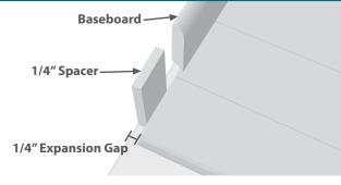
Leave at least 1/4" expansion spaces between flooring and ALL vertical objects (walls, cabinets, pipes, etc.) Large flooring runs may require additional expansion space. Undercut door jambs and casings to provide adequate expansion space. Bamboo Design does not recommend screwing or nailing cabinetry or other permanent fixtures to the flooring.
