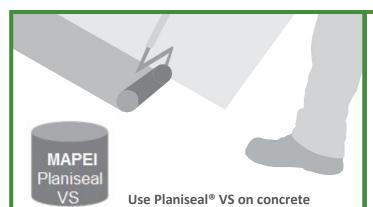
Make sure the subfloor is flat, level, clean and free of debris. New concrete must be cured for at least 60 days. Test the subfloor moisture prior to installation and apply an appropriate moisture barrier such as Mapei Planiseal® on concrete subfloors.
