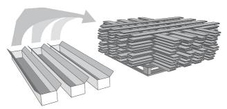
Acclimate your Solid flooring for at least 7 days Cross-stack flooring on a pallet, mixing boards from each box. Acclimate your floor as close to the installation area as possible, for at least 7 days in normal living conditions. More time is necessary in extreme climates.
