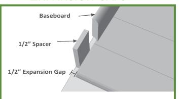
Leave at least 1/2" expansion spaces between flooring and ALL vertical objects (walls, cabinets, pipes, etc.) Large flooring runs may require additional expansion space. Undercut door jambs and casings to provide adequate expansion space.
